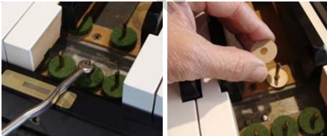
Left: Adjusting a bent oval front rail pin. Right: Adding paper washers to correct the key dip of a black key.
