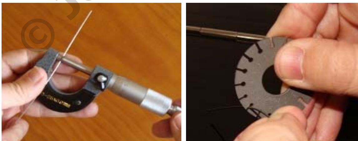
Measuring the diameter of a piano wire using a micrometer or gauge
