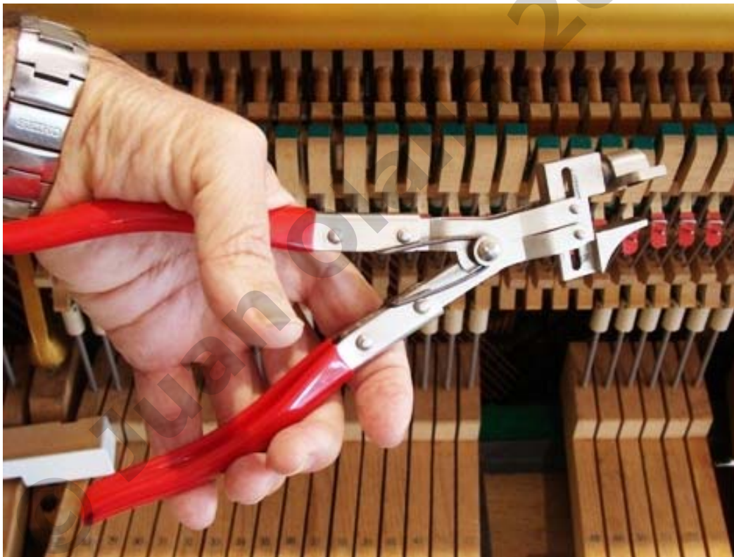
Key easing pliers for squeezing the wood at each side of the bushing and the bushing itself
